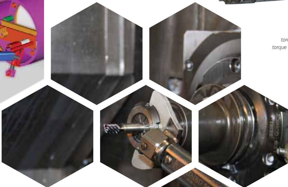
Special fitting for torque tightening of tool collets. Under tightening can result in the collet not holding the tool whereas over tightening can cause damage to the collet.
