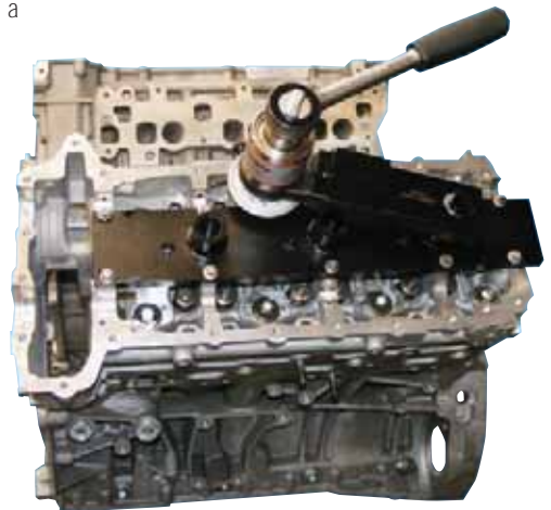
Handtorque multiplier fitted with torque bar adaptor, special torque reaction arm and angle gauge assembly
