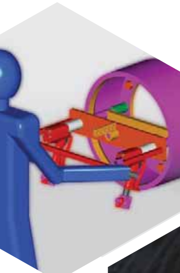
Twin spindle unit comprising of a Pneutorque® stall tool, special nose extensions, reaction plates and frame
