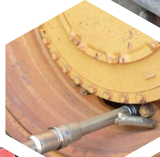
Wheel bolting with Pneutorque® PTM-72
